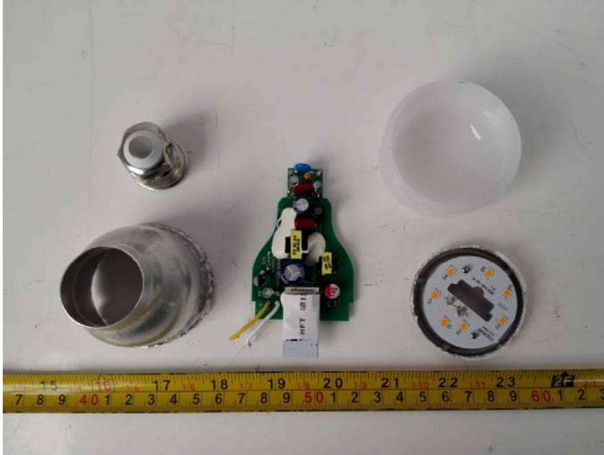
EUT -Cover off View -1
