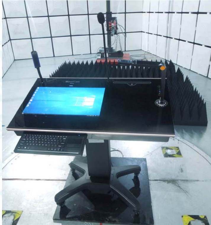
Photo of Setup for Radiated Emission (Below 1 GHz)
