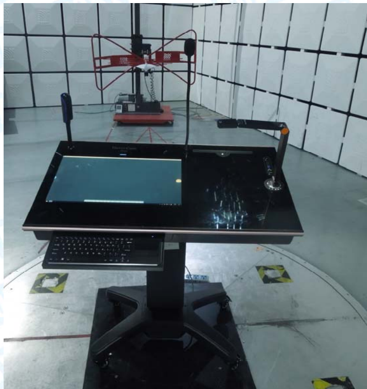
Photo of Setup for Radiated Emission (Below 1 GHz)
