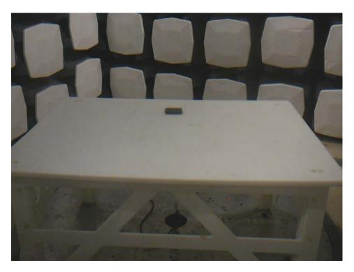
13.2 Radiated Emission below 1 GHz Rear View at 3 Meters
