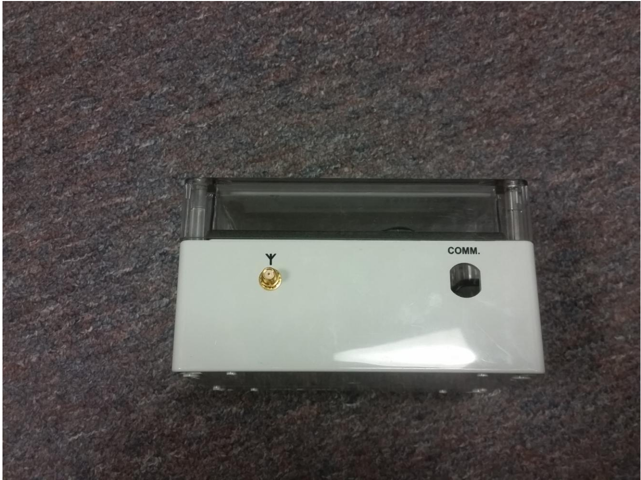
** Note: COMM. Port connector hole was for prototyping only
