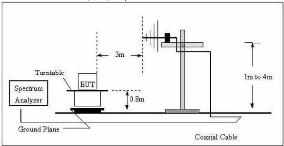
(C) Radiated Emission Test-Up Frequency Above 1GHz
