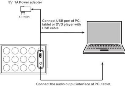
Connect the audio output interface of PC, tablet, mobile phone, Mp3, Mp4, etc with line-in cable
