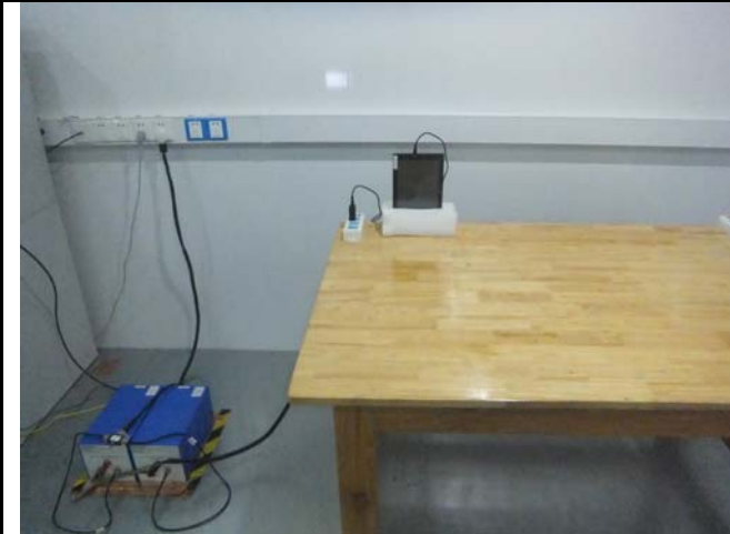
Conducted Emissions Test Setup Front View
