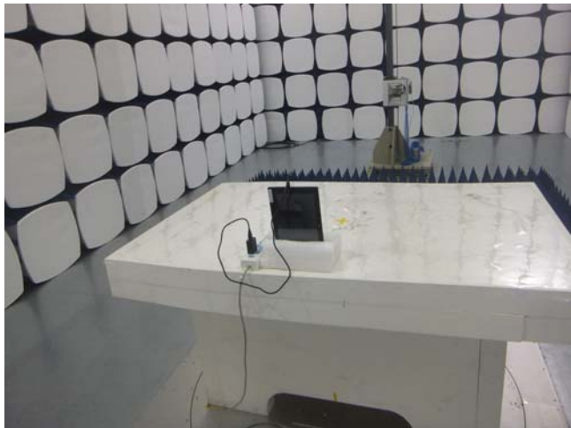
Conducted Emissions Test Setup Front View
