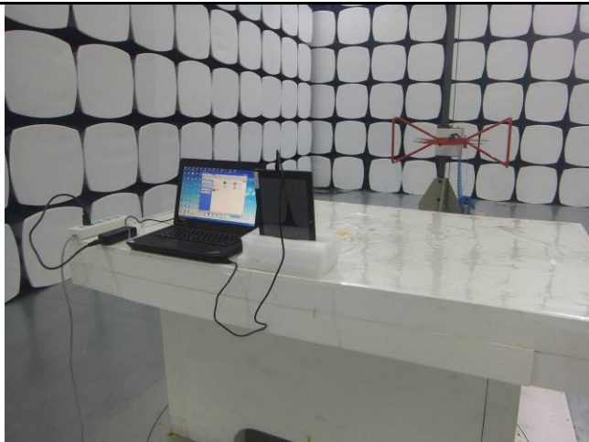
Conducted Emissions Test Setup – Front View
