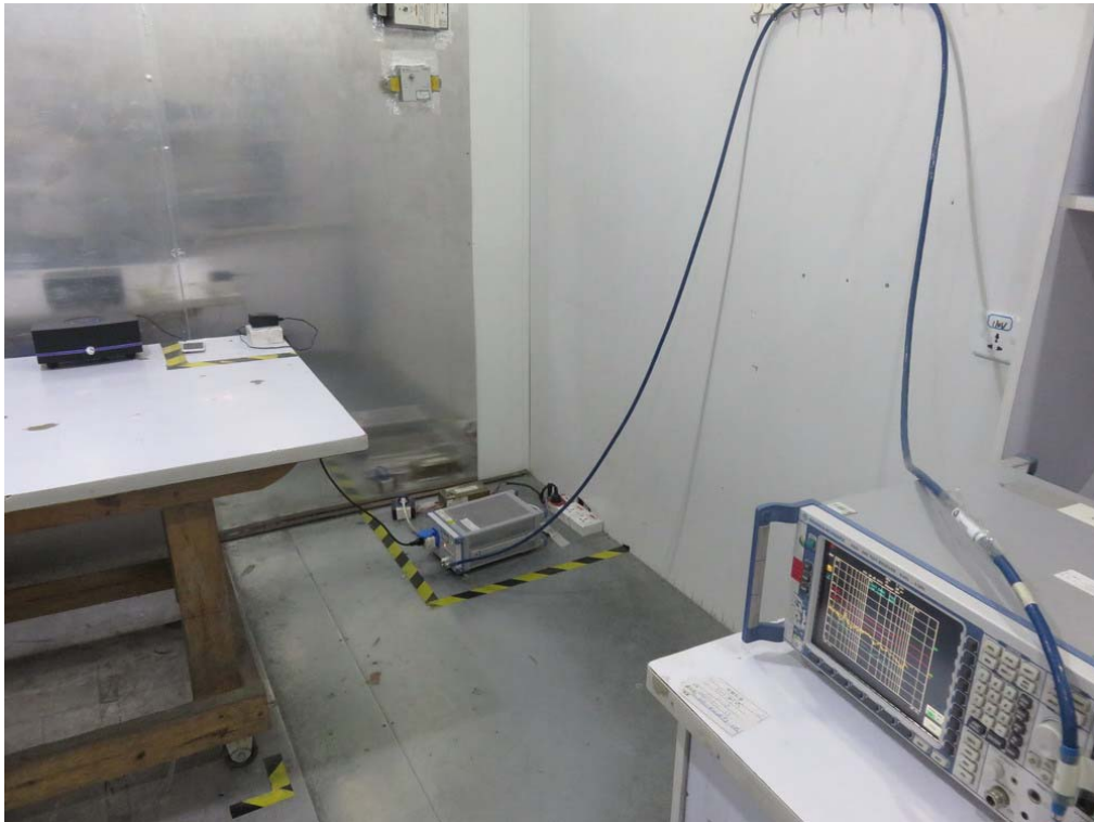
FCC RADIATED EMISSION TEST SETUP
