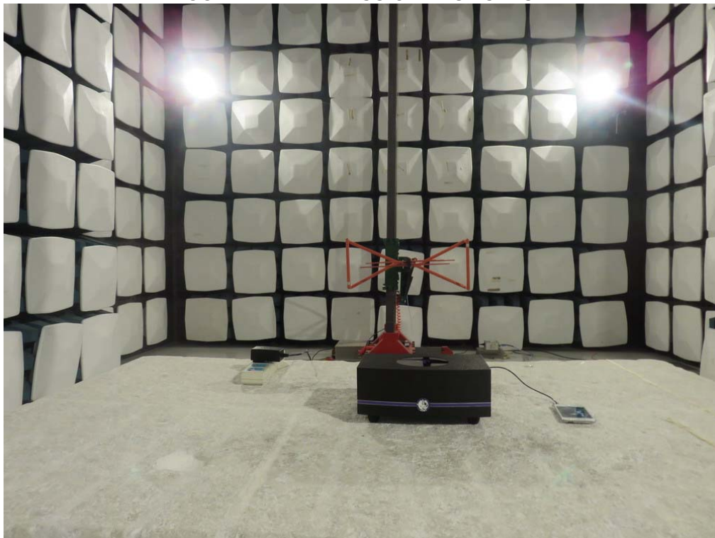
FCC RADIATED EMISSION TEST SETUP
