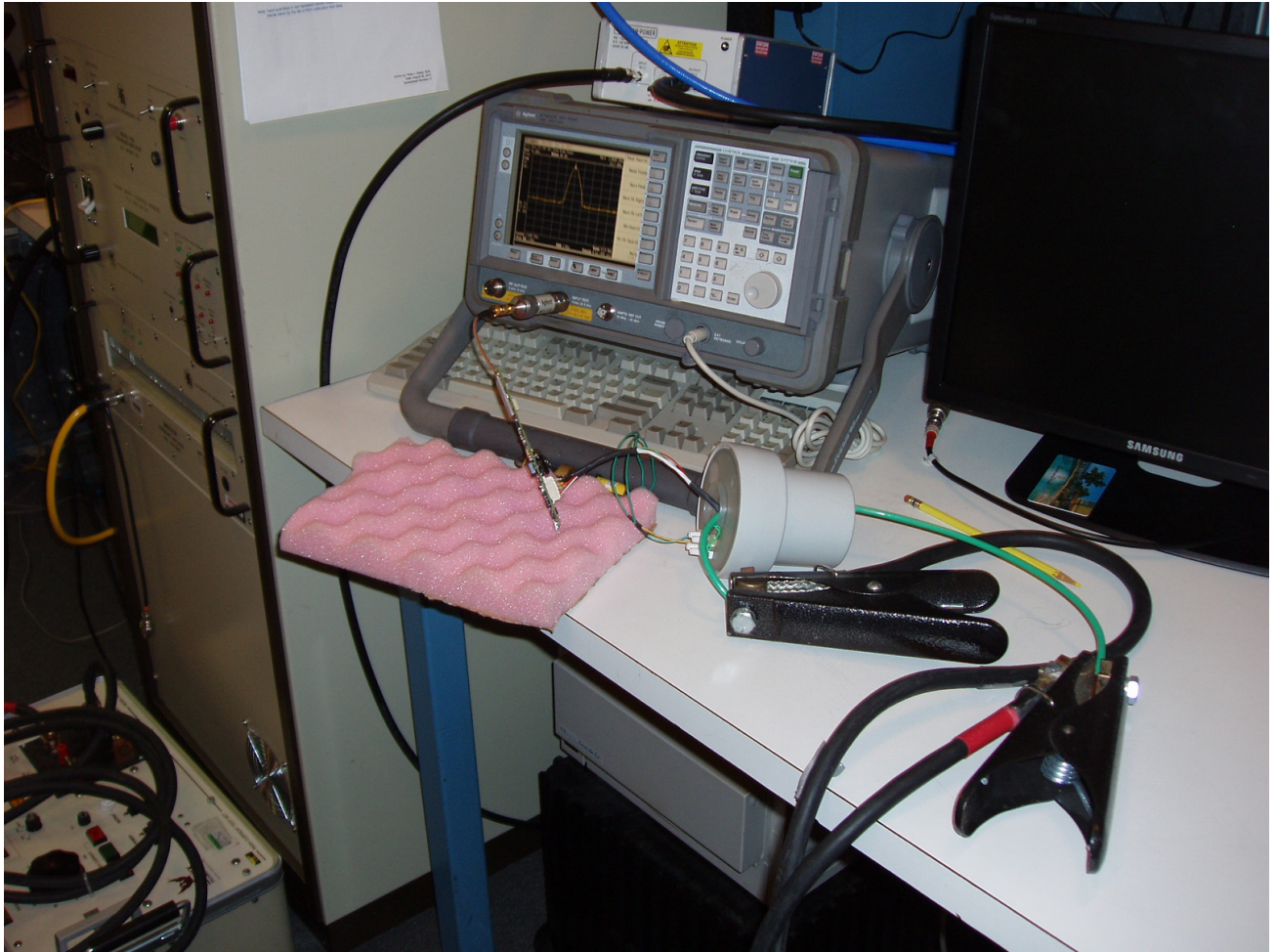
Photo 4 – Antenna Port Conducted Test Set-up
