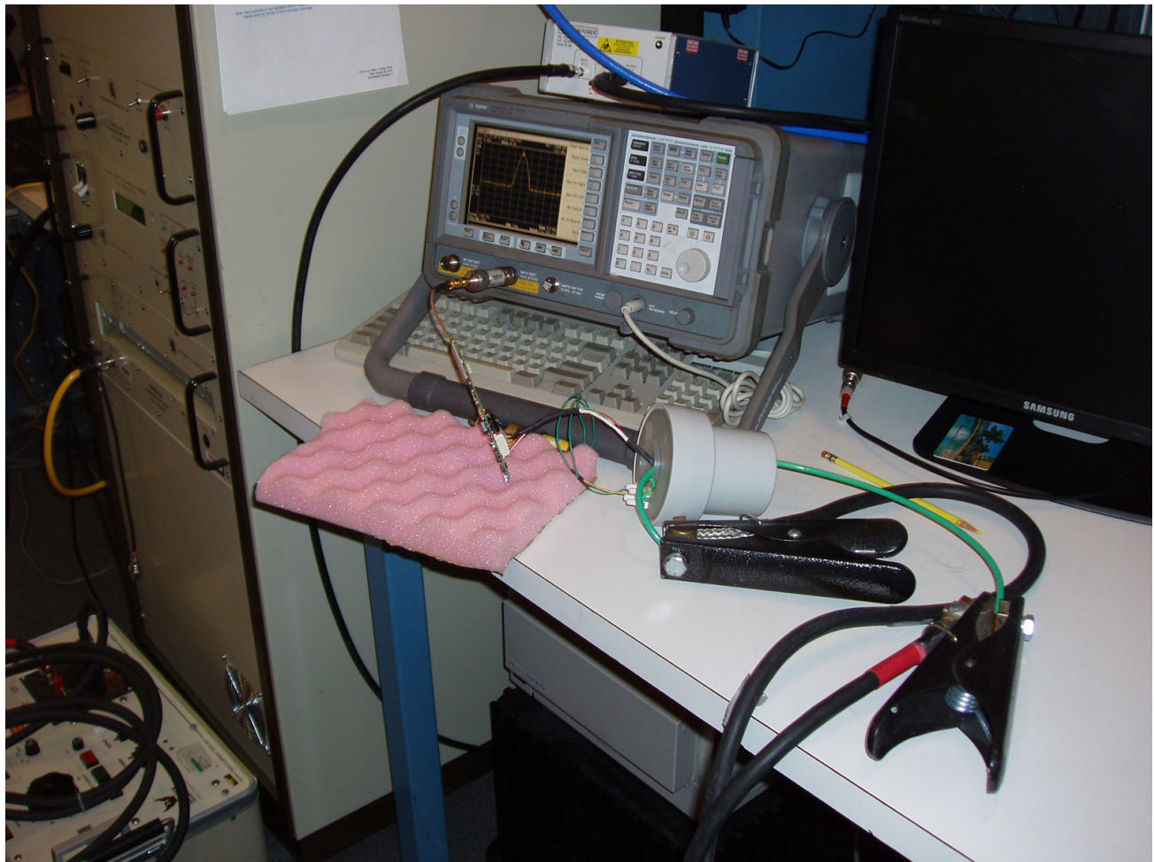
Photo 7.4-1 – Conducted Measurement Test -Setup
