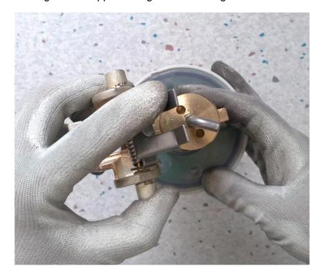
Turn the tripping pin 90°, until the lower contact is firmly blocked.
