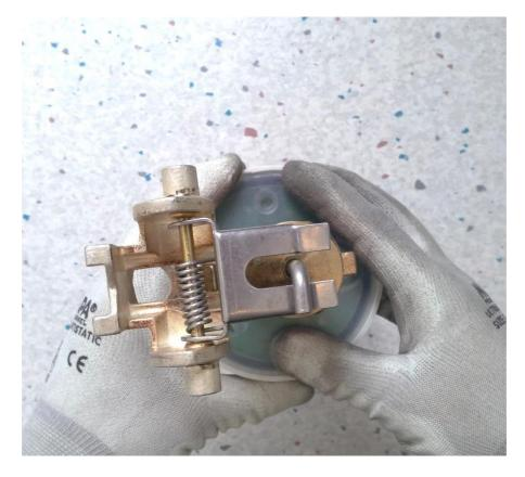
Place the pole in the tube inferior eyelet and position in the cutout-base.
