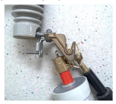
Withdraw the pole and place it in the tube's superior eyelet. Push it until it remains in closing position.
