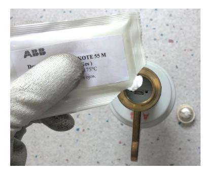
Check the condition of the O-Ring and apply silicon grease both inside the cap and over the micro-USB connector.
