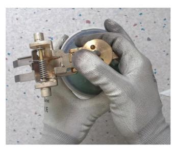
Turn the tensioning device support.
