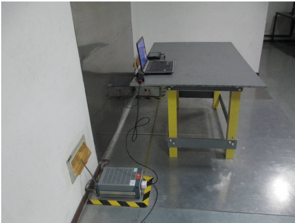
Conducted Emissions Test Setup Side View
