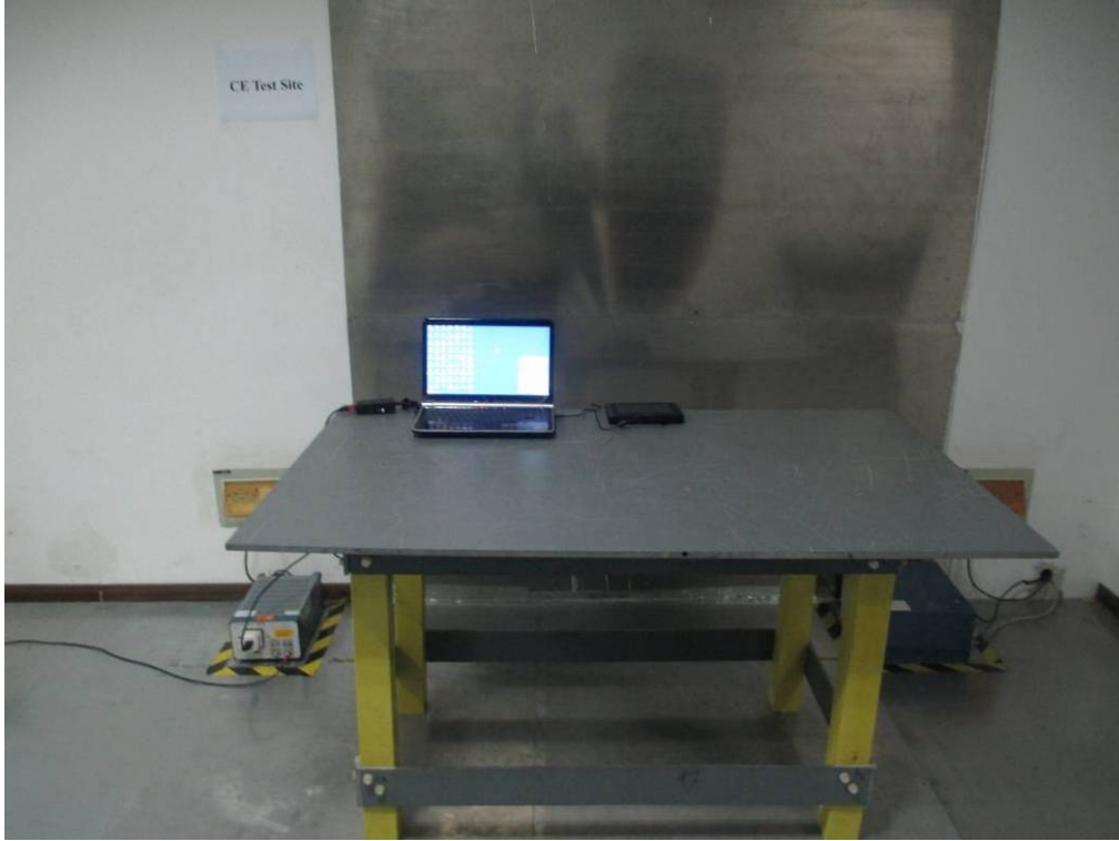
Conducted Emissions Test Setup Front View
