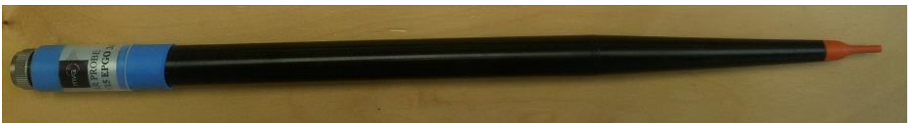
Figure 1 – MVG COMOSAR Dosimetric E field Dipole
