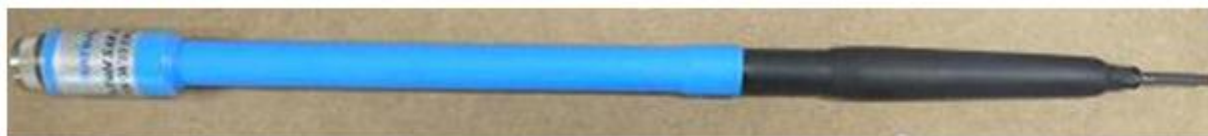
Figure 1 – Satimo COMOSAR Dosimetric E field Dipole
