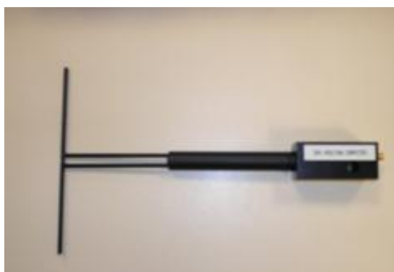
Figure 1 – Satimo COMOSAR Validation Dipole
