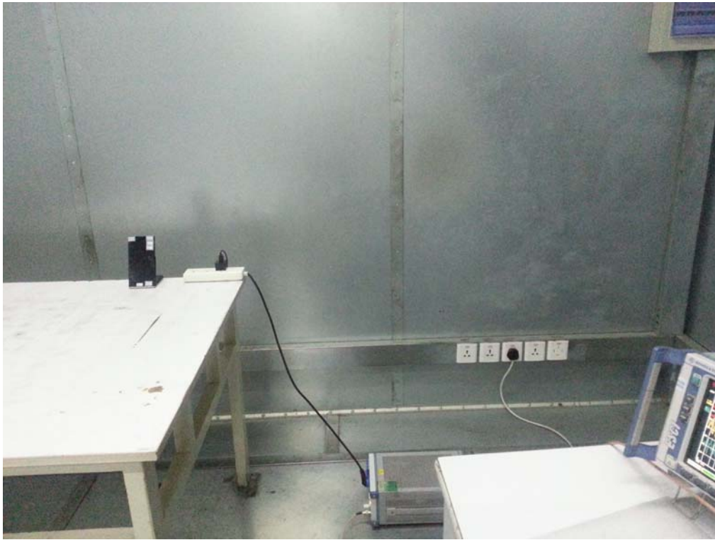
Set-up for Conducted Emission Test
