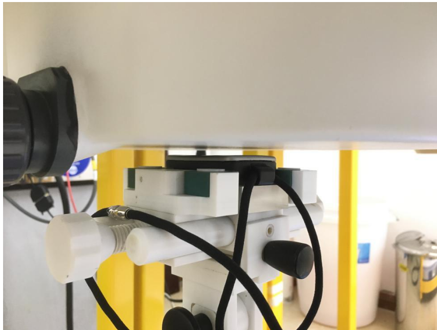
Body worn _ Front with Lanyard (Test distance: 5mm, Thickness of DUT: 16mm)
