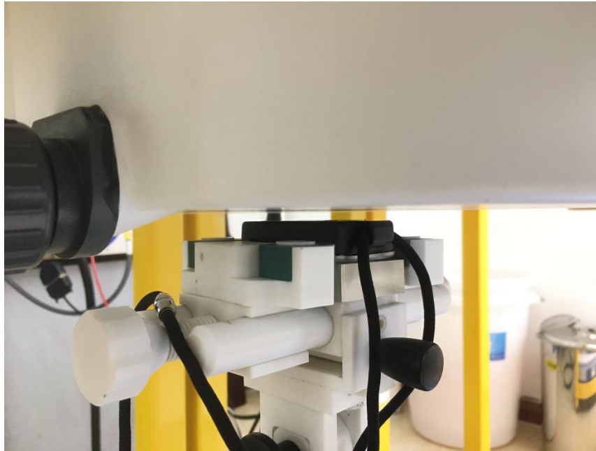
Body worn _ Back With Lanyard (Test distance: 5mm, Thickness of DUT: 16mm)
