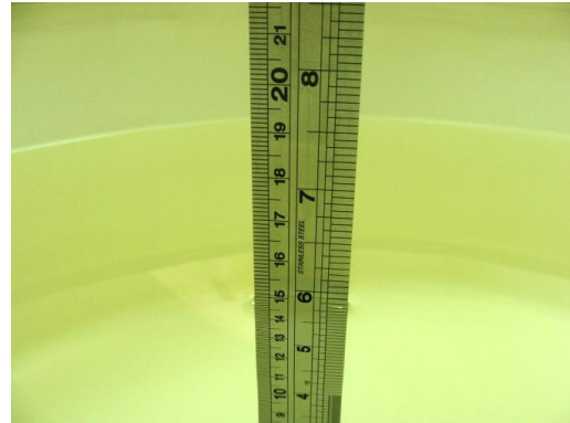
Fig 6.2 Photo of Liquid Height for Body SAR
