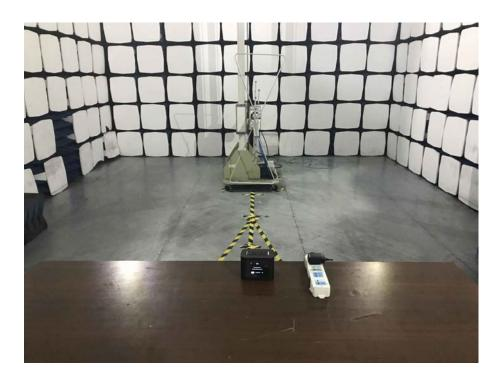
Radiation Emission Test Setup (Above 1GHz)
