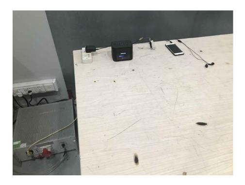
Radiation Emission Test Setup (Below 30MHz)
