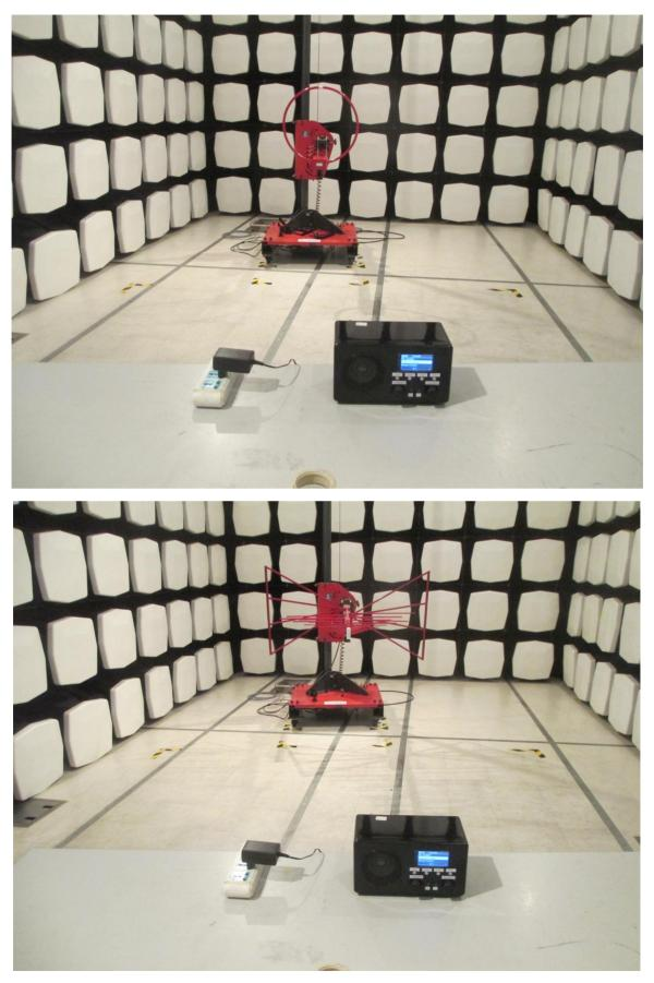
MEASUREMENT OF RADIATED EMISSION TEST SET UP
