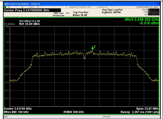
In-Band Reference Level IEEE 802.11g_Channel 6_20MHz_Antenna 0
