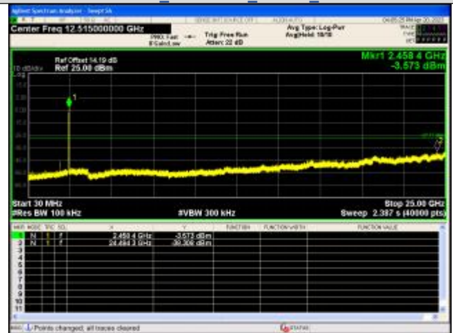
Spurious Emission IEEE 802.11n Channel 9 40MHz Antenna 0
