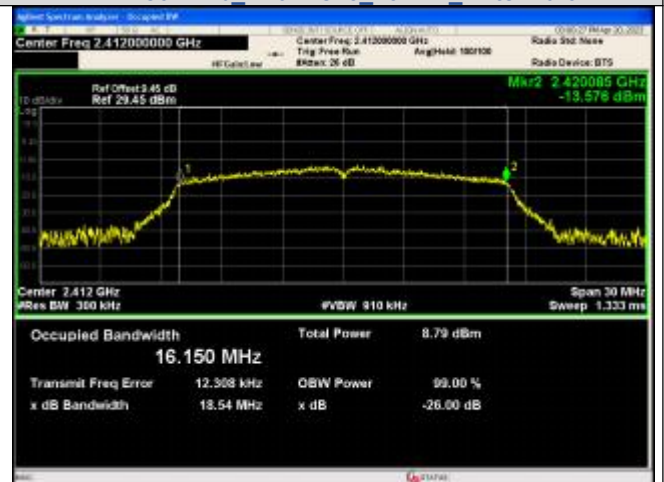
IEEE 802.11g_Channel 1_20MHz_Antenna 0
