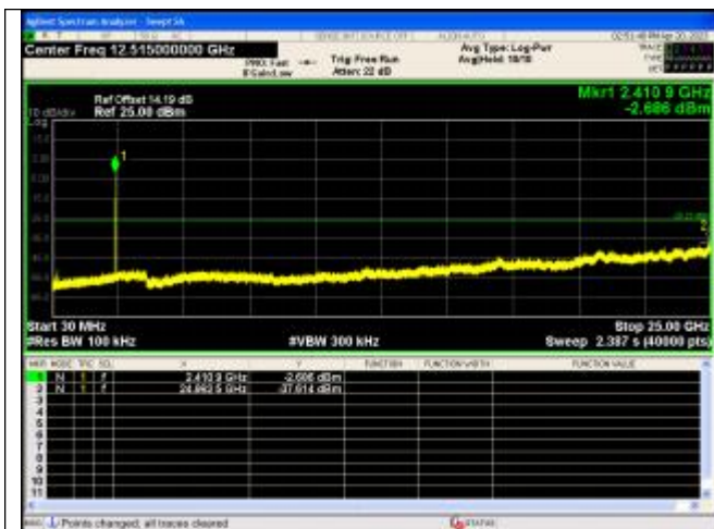
Spurious Emission IEEE 802.11b Channel 1 20MHz Antenna 0
