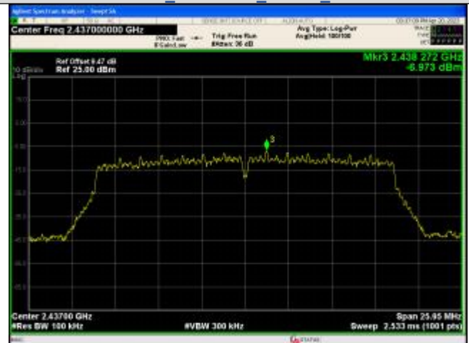
In-Band Reference Level IEEE 802.11n_Channel 6_20MHz_Antenna 0
