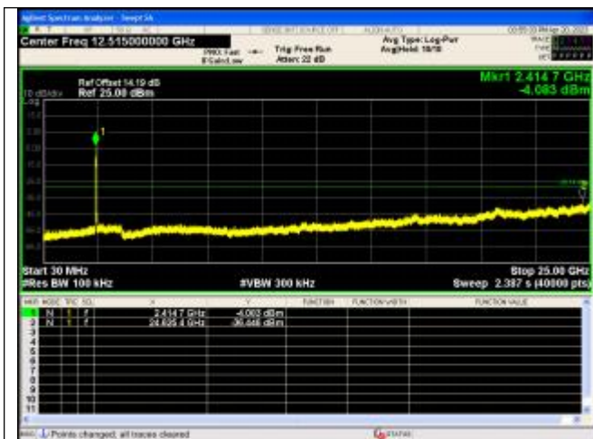
Spurious Emission IEEE 802.11n Channel 3 40MHz Antenna 0
