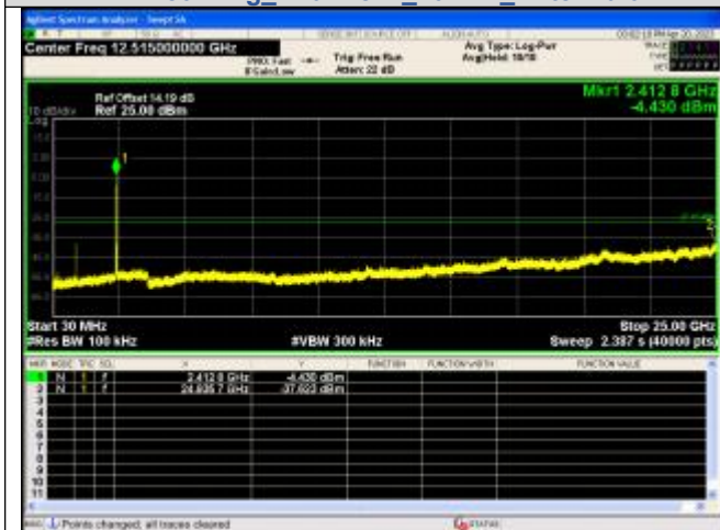
Spurious Emission IEEE 802.11g Channel 1 20MHz Antenna 0
