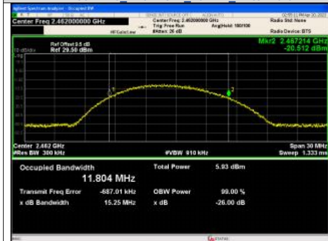
IEEE 802.11b_Channel 11_20MHz_Antenna 0
