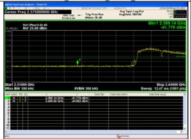
Out Of Band Emission IEEE 802.11n_Channel 3_40MHz_Antenna 0
