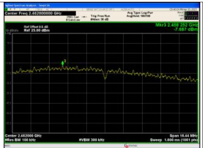
In-Band Reference Level IEEE 802.11n_Channel 11_20MHz_Antenna 0
