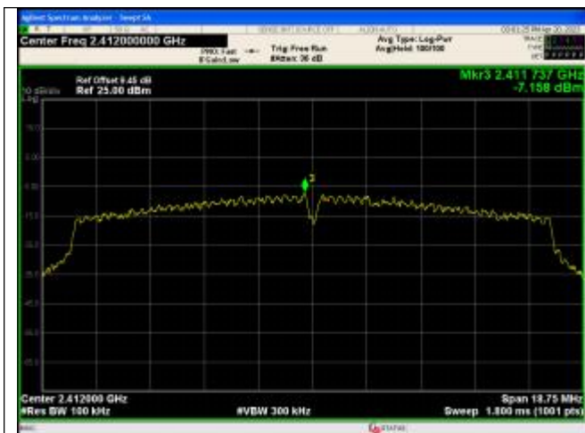
In-Band Reference Level IEEE 802.11g Channel 1 20MHz Antenna 0
