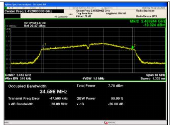
IEEE 802.11n_Channel 9_40MHz_Antenna 0
