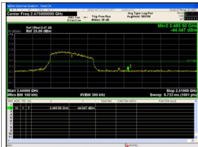
Out Of Band Emission IEEE 802.11g_Channel 11_20MHz_Antenna 0
