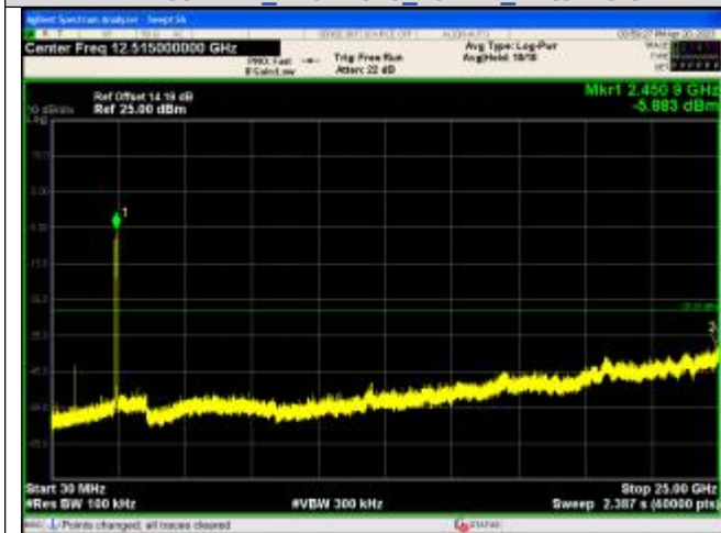
Spurious Emissions IEEE 802.11n Channel 6 40MHz Antenna 0
