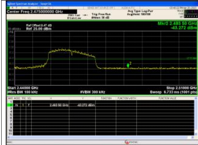
Out Of Band Emission IEEE 802.11n_Channel 11_20MHz_Antenna 0
