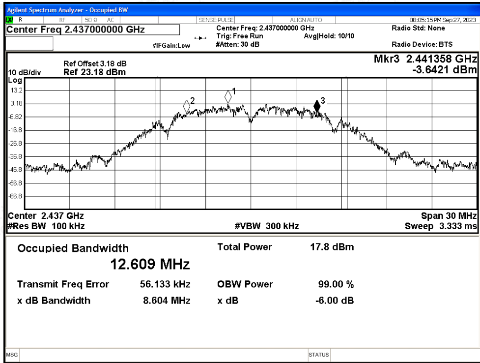
-6dB Bandwidth NVNT b 2437MHz Ant1
