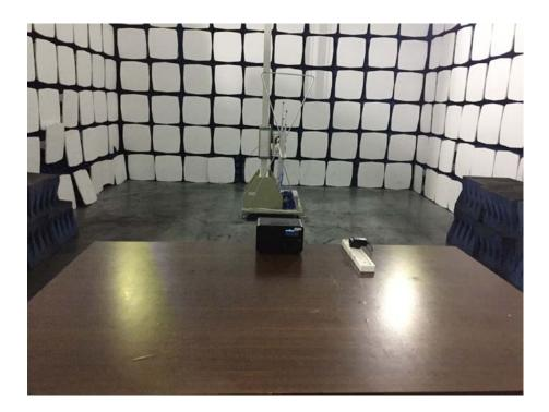
Radiation Emission Test Setup (Above 1GHz)
