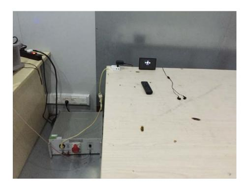
Radiation Emission Test Setup (Below 30MHz)
