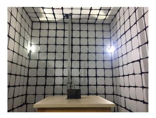
Radiation Emission Test Setup (Above 1GHz)
