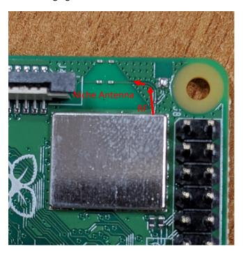
Niche Antenna on board connected to the passive RF switch (Skyworks Part number SKY13351-378LF), switch directly connected to the Module. You must follow the design guidelines for the antenna.
