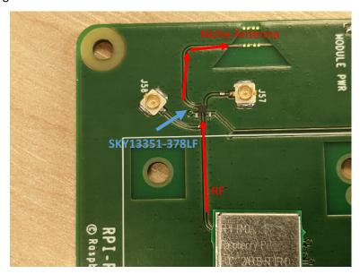
Antenna (Manufacturer; Raspberry Pi Part number YH2400-5800-SMA-108) connected to UFL connector (Taoglas RECE.20279.001E.01) connected to RF switch (Skyworks Part number SKY13351-378LF) directly connected to the RM0 module. Photo shown below
