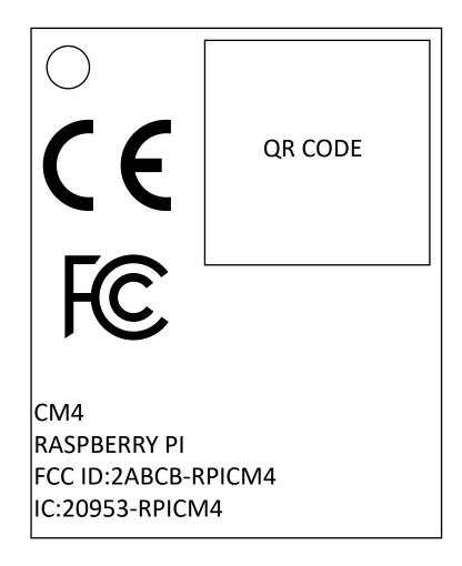
All label markings are Laser etched on top of RF shield at production
