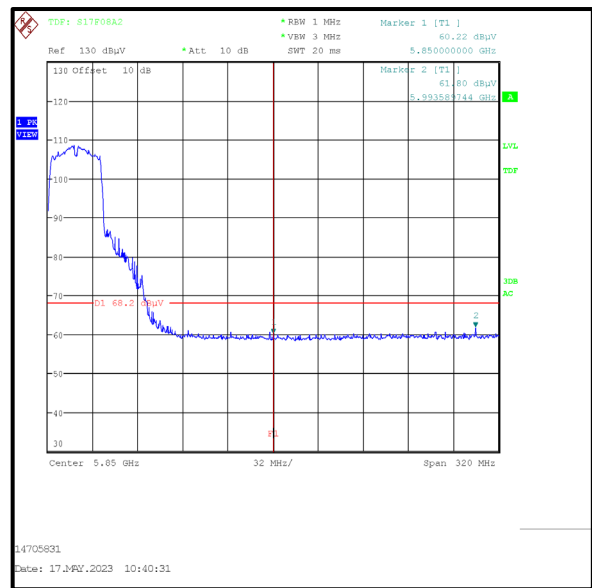
Straddle Channel emission level at 5850 MHz
