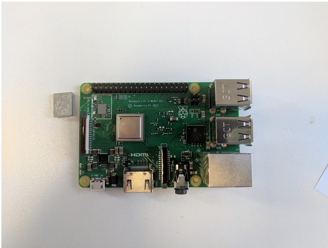
Front of PCB with RF shield removed
