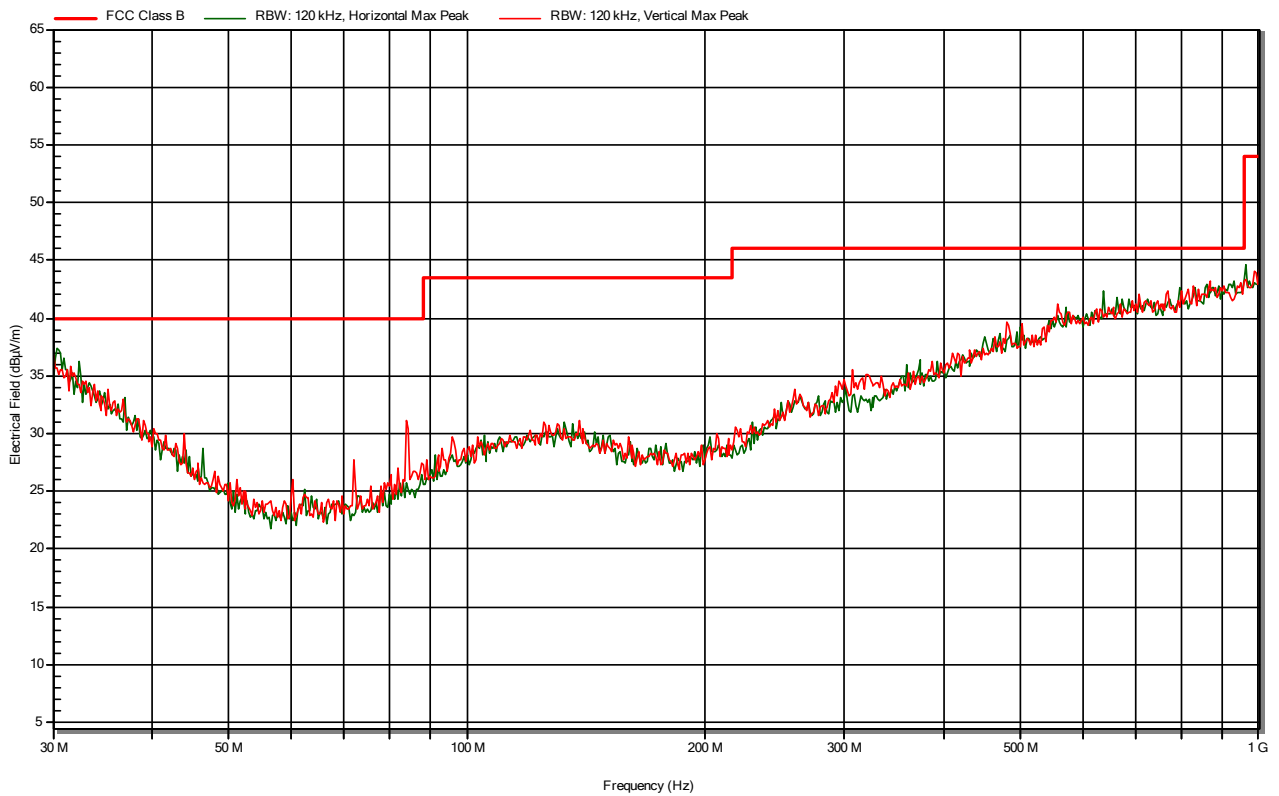
Figure 5.3.7.3: Electric field emissions Plot IEEE 802.11b, 30MHz to 1GHz, Operation on 2462MHz - Peak detector scan
