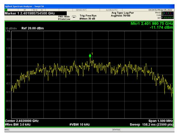
Figure 8.2.6.1 Power spectral density, Operation on channel 2402MHz
