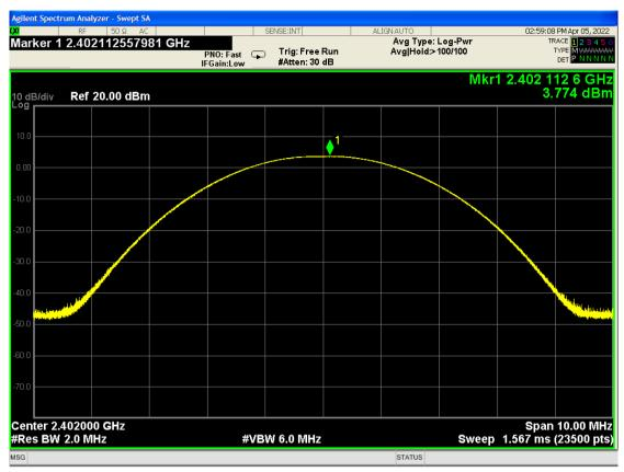
Figure 7.2.6.1 Peak output power, Operation on channel 2402MHz
