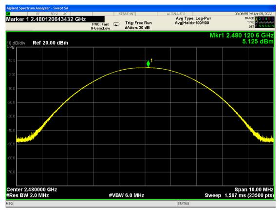
Figure 7.2.6.3 Peak output power, Operation on channel 2480MHz
