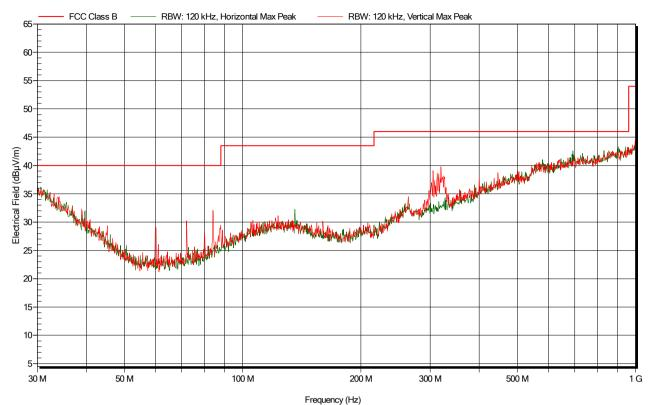
Figure 5.3.7.2: Electric field emissions Plot, 30MHz to 1GHz, Operation on 2402MHz - Peak detector scan
