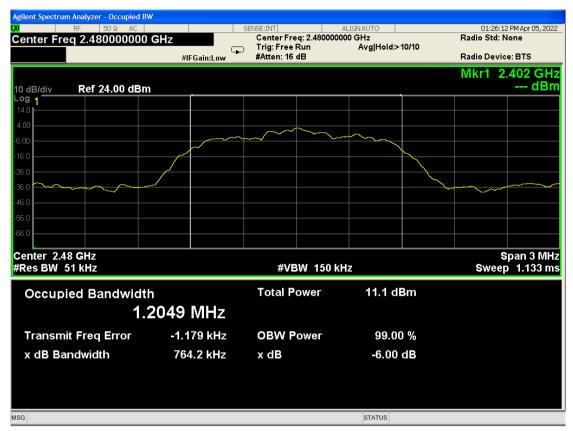
Figure 6.2.6.3 Bandwidth at 6dB Point and 99% Occupied Bandwidth. Operation on channel 2480MHz
