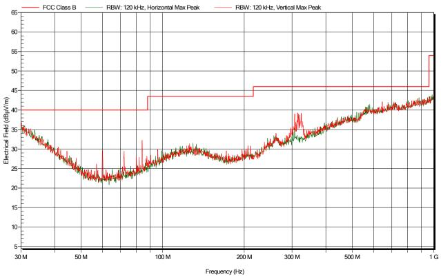
Figure 5.3.7.3: Electric field emissions Plot, 30MHz to 1GHz, Operation on 2440MHz - Peak detector scan
