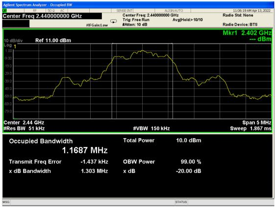
Figure 6.2.6.2 Bandwidth at 20dB Point and 99% Occupied Bandwidth. Operation on channel 2440MHz
