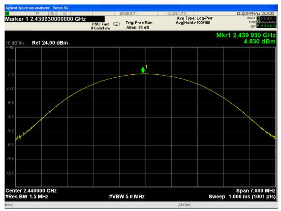
Figure 7.2.6.2 Peak output power, Operation on channel 2440MHz
