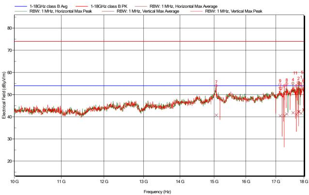
Figure 5.4.9.2: Electric field emissions Plot, 10GHz to 18GHz. 1m measurement distance. Operation on 2440MHz
