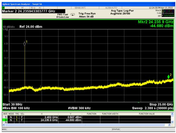
Conducted emissions 30MHz to 25GHz. Operation on channel 2402MHz.
