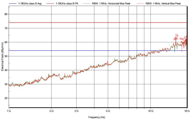
Figure 5.4.9.4: Electric field emissions Plot, 1GHz to 18GHz, Operation on 2480MHz – Peak detector scan
