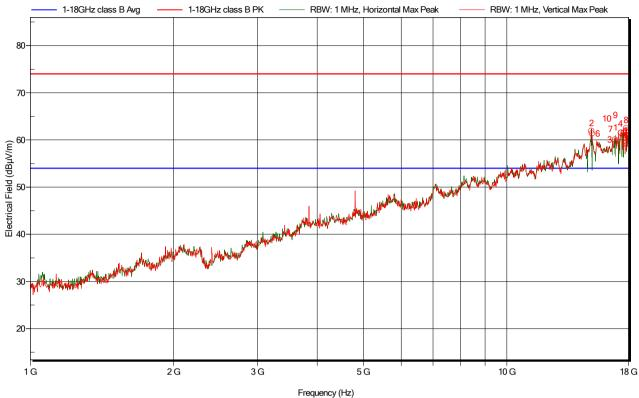
Figure 5.4.9.3: Electric field emissions Plot, 1GHz to 18GHz, Operation on 2402MHz - Peak detector scan
