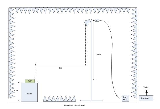
Figure 5.4.7.1: Test Setup for Final E-Field Measurements from 1GHz to 18GHz
