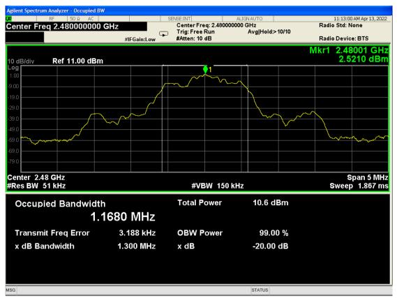
Figure 6.2.6.3 Bandwidth at 20dB Point and 99% Occupied Bandwidth. Operation on channel 2480MHz
