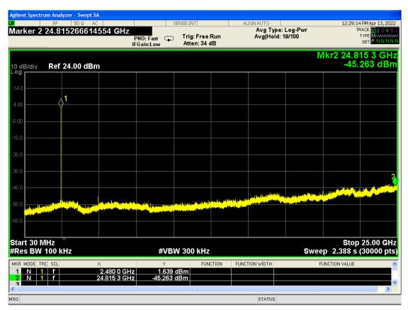
Conducted emissions 30MHz to 25GHz. Operation on channel 2480MHz.
