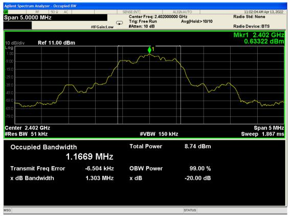
Figure 6.2.6.1 Bandwidth at 20dB Point and 99% Occupied Bandwidth. Operation on channel 2402MHz
