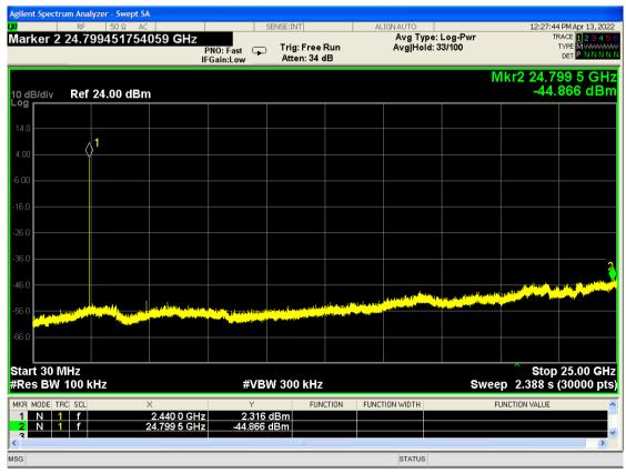
Conducted emissions 30MHz to 25GHz. Operation on channel 2440MHz.
