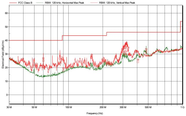
Figure 5.3.7.1: Electric field emissions Plot, 30MHz to 1GHz, 2480MHz Operation
