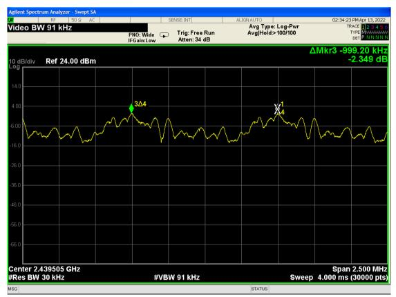
Figure 8.2.7.1: Carrier frequency separation
