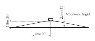
Note: Attention detection beams go across access points such as windows, doors during sensor installation.
