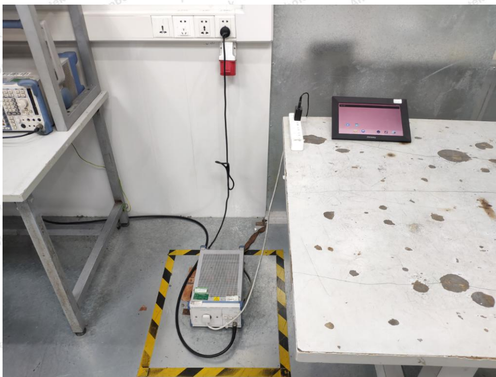
Photo of Power Line Conducted Emission Test
