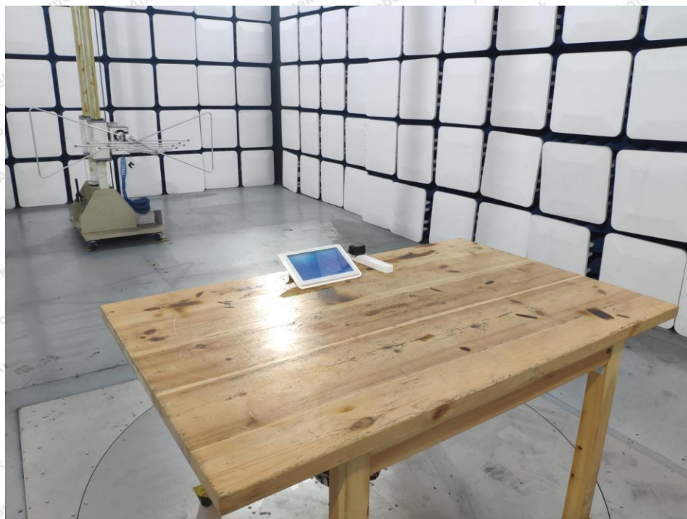
Photo of Radiation Emission Test
