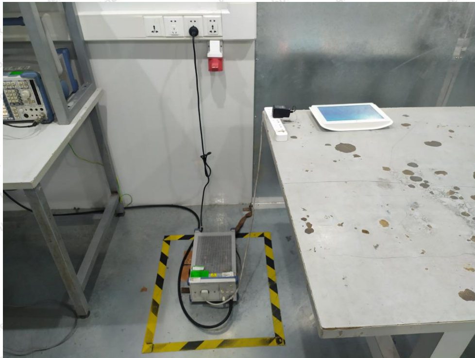
Photo of Power Line Conducted Emission Test
