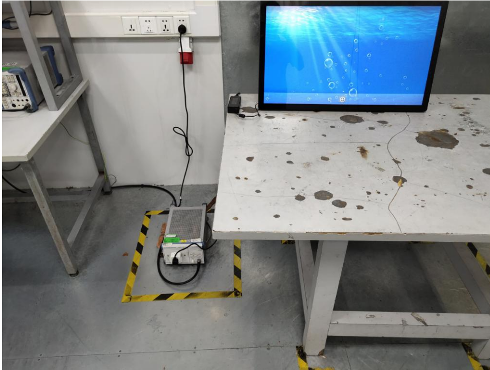
Photo of Power Line Conducted Emission Test
