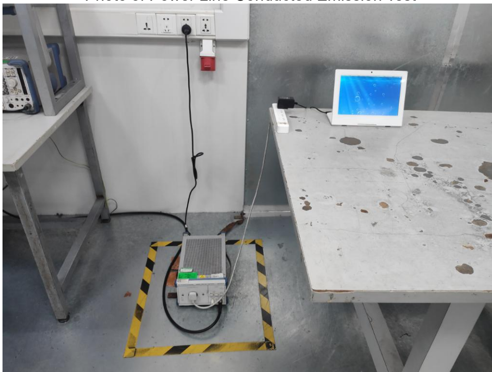
FCC ID: 2ABC5-WL1012T Photo of Power Line Conducted Emission Test
