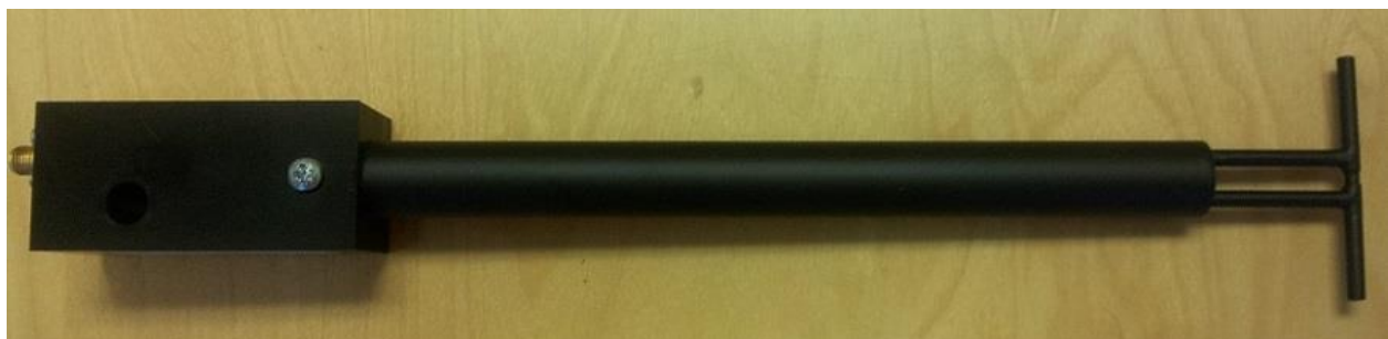
Figure 1 – MVG COMOSAR Validation Dipole
