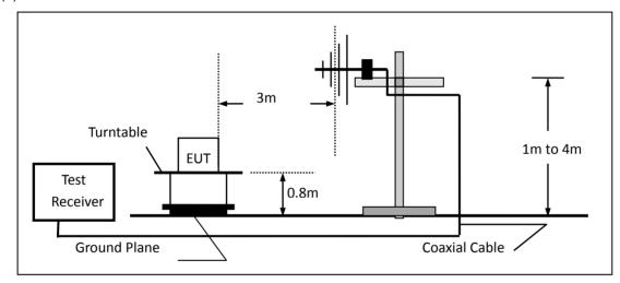
(c) For radiated emissions above 1000MHz
