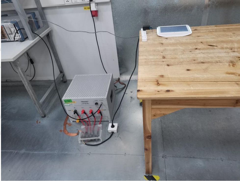
Photo of Conducted Emission Measurement
