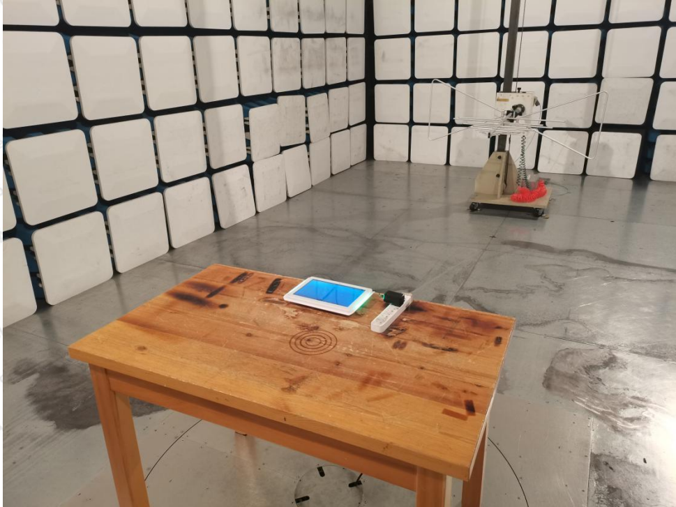
Photo of Radiation Emission Test
