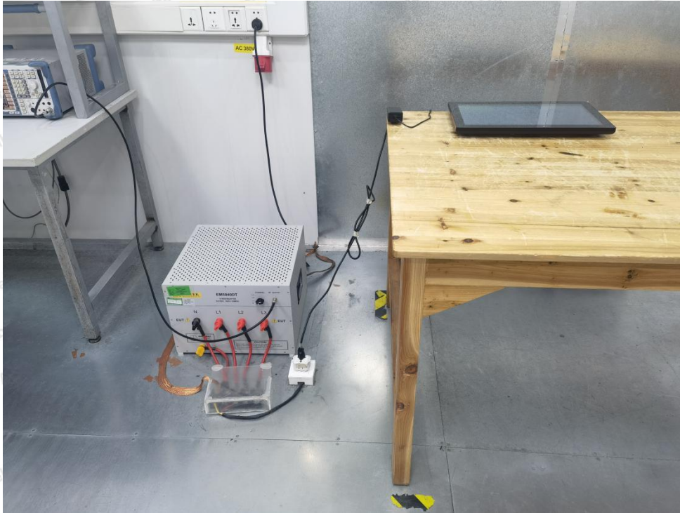
Photo of Conducted Emission Measurement
