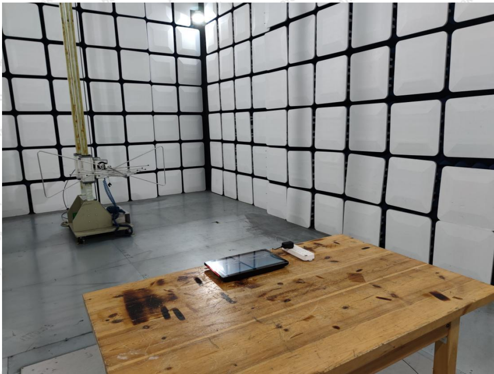
Photo of Radiation Emission Test
