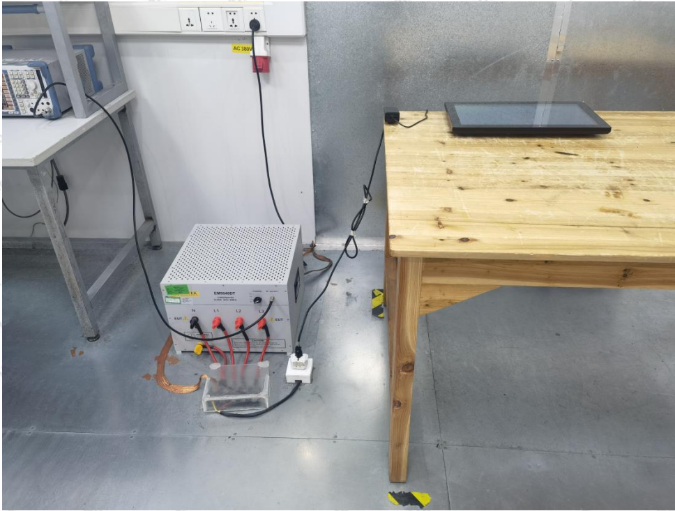
Photo of Conducted Emission Measurement
