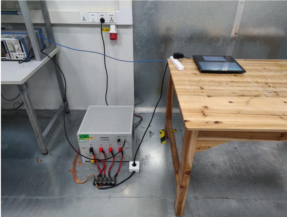
Photo of Conducted Emission Measurement
