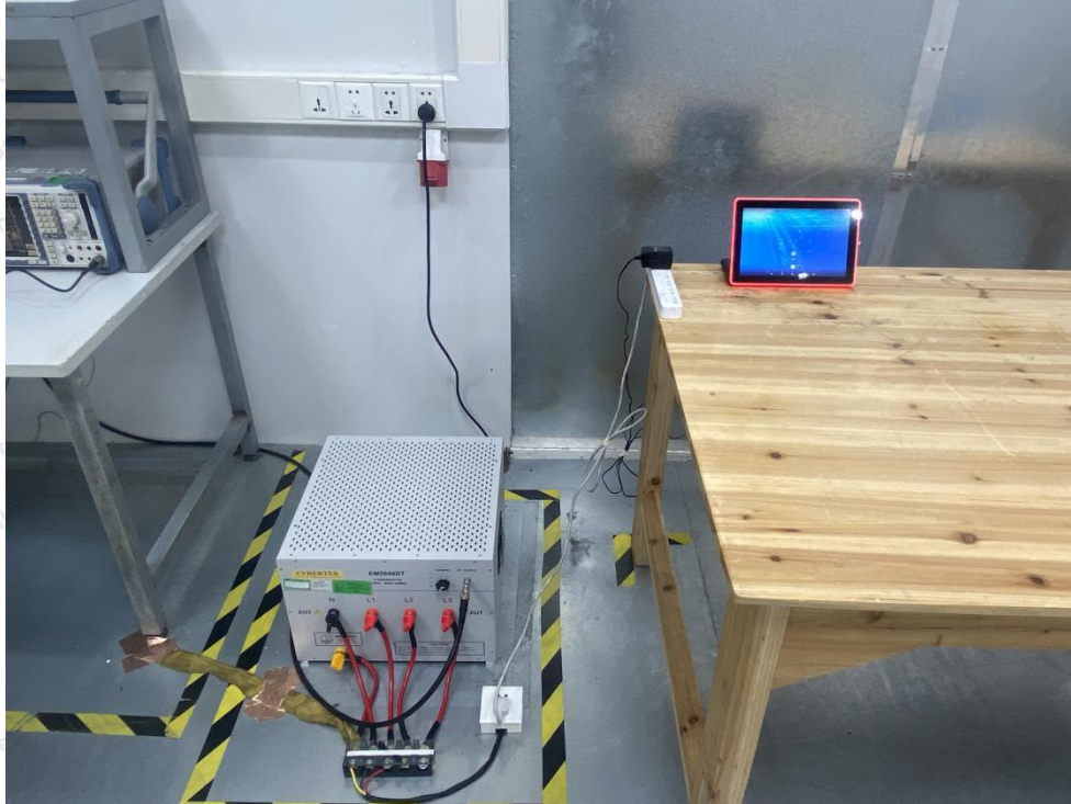
Photo of Conducted Emission Test
