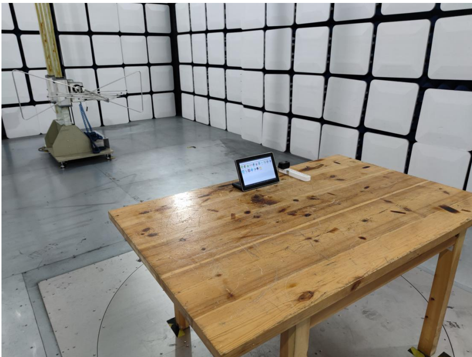
Photo of Radiation Emission Test
