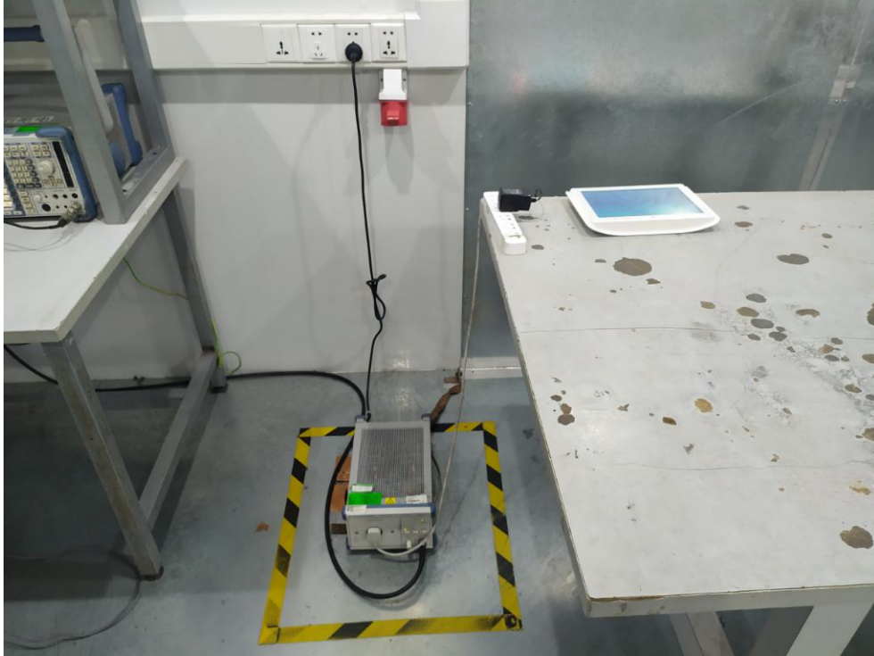
Photo of Power Line Conducted Emission Test
