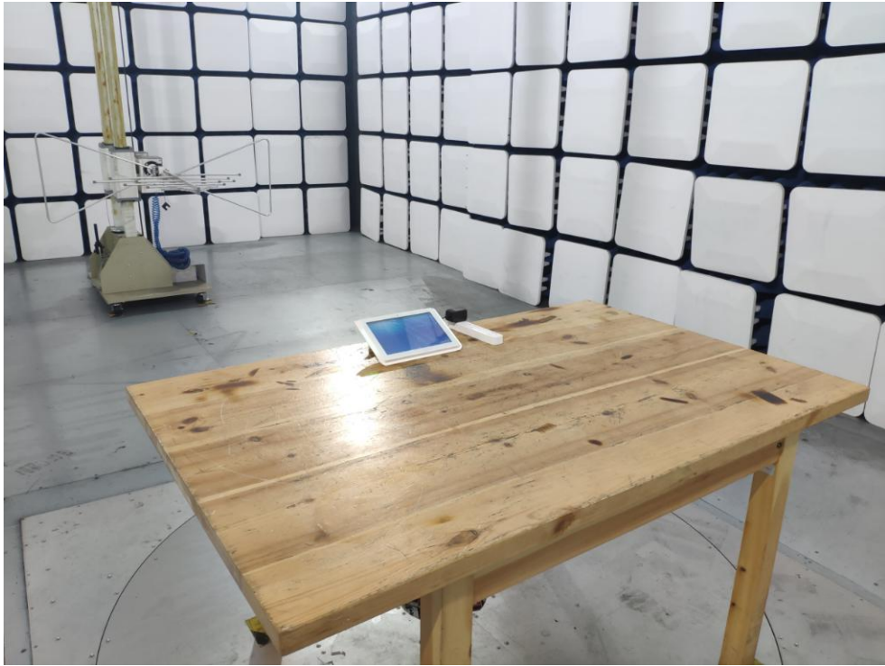
Photo of Radiation Emission Test
