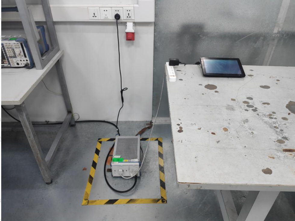
Photo of Power Line Conducted Emission Test
