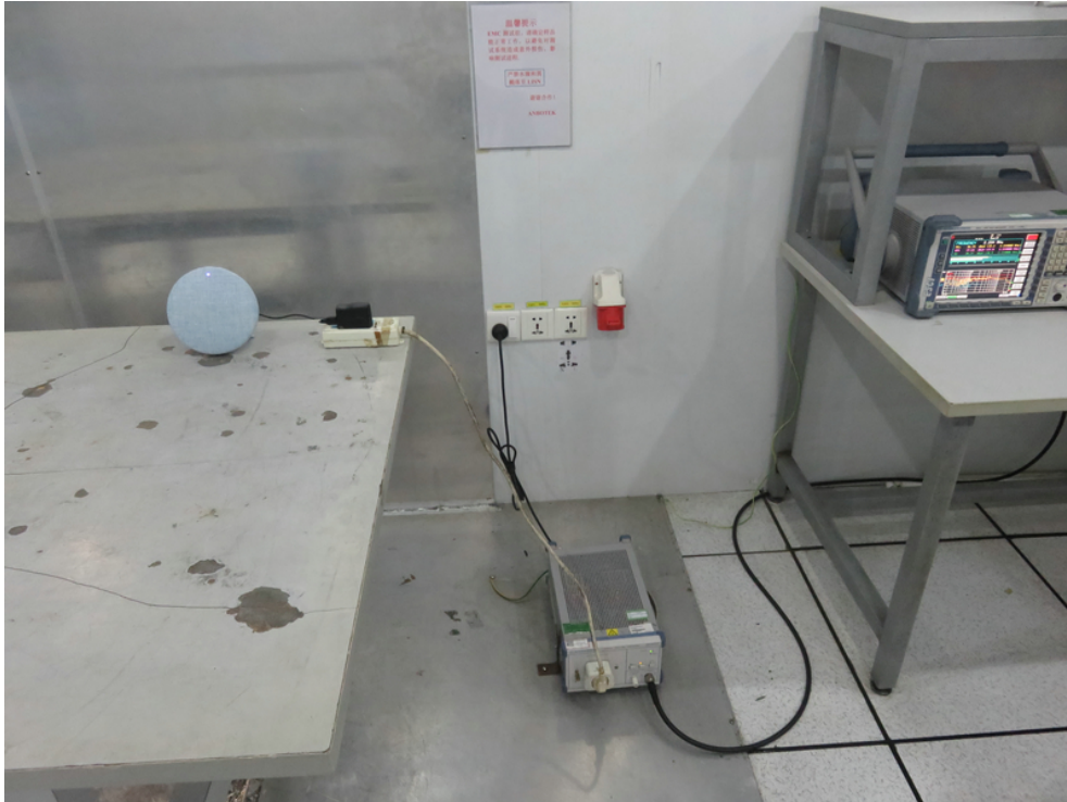
Photo of Conducted Emission Measurement
