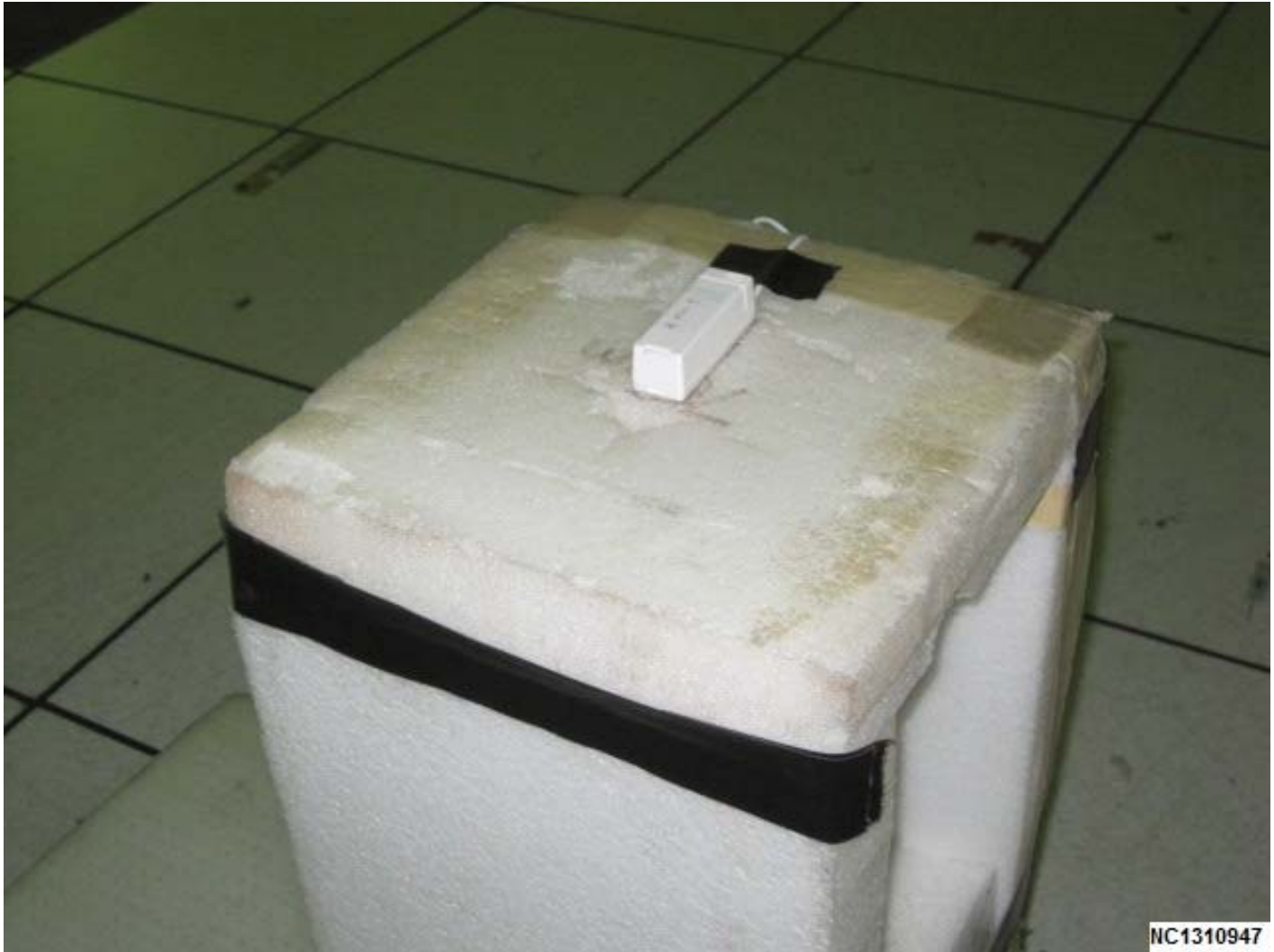
Test-setup photo(s): radiated emissions
